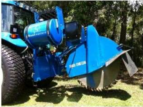
Image 47: Root pruning is done with a large blade attached to the back of a tractor that drives slowly down the rows and cuts down into the soil.
