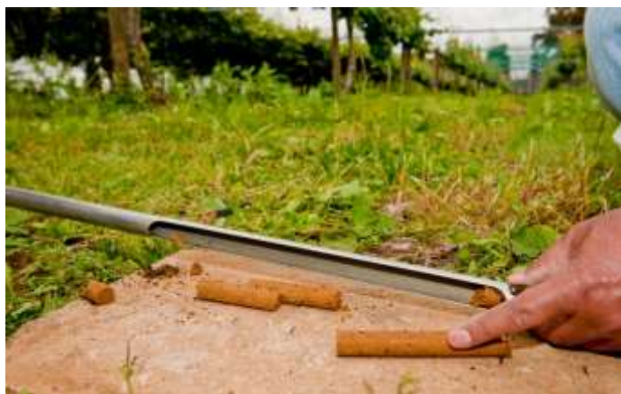
Image 7: Measuring the carbon in soil on an orchard (J Troughton).
