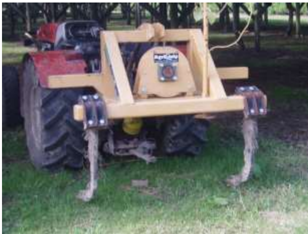
Image 48: Ripper attached to the back of a tractor, used to help improve soil drainage (Shane Max).
